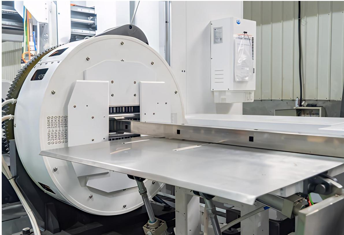
The **platform servo support system** is designed to enhance automation, precision, and efficiency in tube laser cutting operations. It enables **automatic transfer of cut workpieces** to the designated collection area, while a **waste box is positioned directly beneath the cutting zone** to collect scrap material efficiently.
