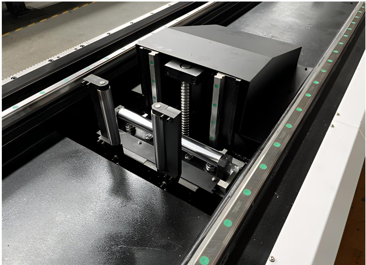
The **servo floating follow-up support** is engineered to provide intelligent, adaptive support for pipes and profiles during laser cutting. It **automatically follows the vertical movement** of the material in real time, eliminating the need for manual adjustment and ensuring the pipe remains **self-centered** throughout the cutting process.
