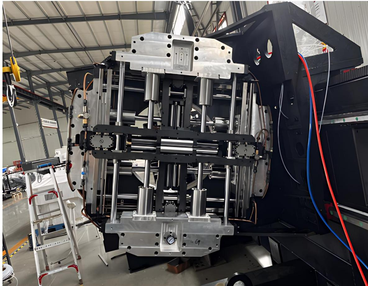
The patented front-mounted full-stroke pneumatic chuck is engineered for high-performance tube and profile clamping in industrial laser cutting systems. Featuring a **square-through-hole design**, it offers enhanced material pass-through capability, making it suitable for a wide range of profile types.
