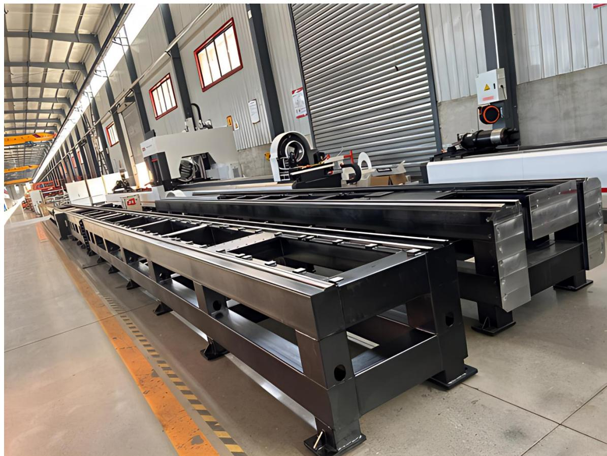
The machine bed is **welded using high-quality raw materials** and undergoes a rigorous multi-stage treatment process to ensure structural integrity and long-term performance. This includes **stress relief annealing** after rough machining, followed by **secondary vibration aging treatment**, and final **precision machining on a large-scale gantry milling center**.
