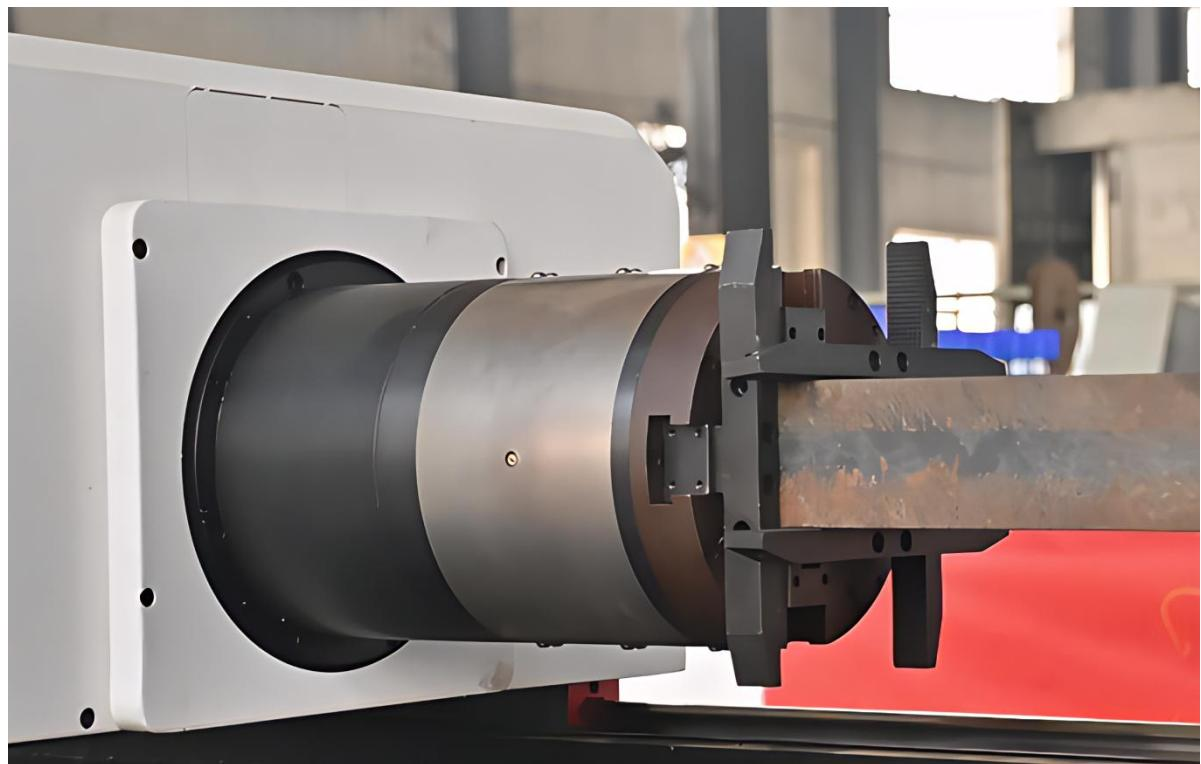
The full-stroke pneumatic rear chuck is designed for high-speed, high-precision tube clamping with built-in **buffering technology** to ensure zero damage to workpieces during operation. With a **maximum rotation speed of 85 r/min**, it supports efficient and stable processing across a wide range of applications.
