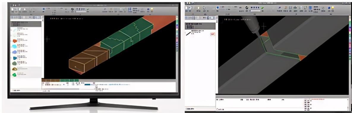
The **FSCUT TubesT Nesting System** is a powerful and intelligent software solution designed specifically for tube laser cutting. It supports both **single-part and multi-part nesting**, maximizing material utilization and minimizing waste through optimized layout strategies.
