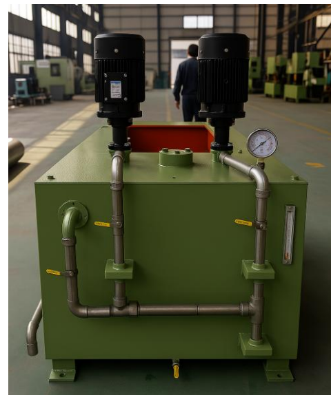
Emulsion Cooling System
