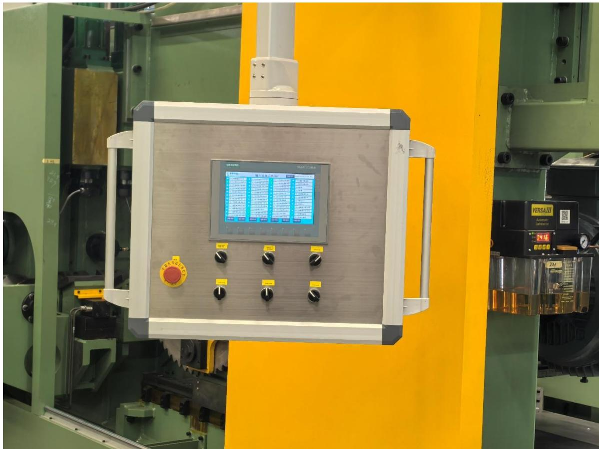
The system adopts Siemens S7-1500 series PLC as the core control platform, integrated with the latest generation servo drive system and G120 inverter to achieve precise control of saw blade feed, spindle speed, and auxiliary operations.
