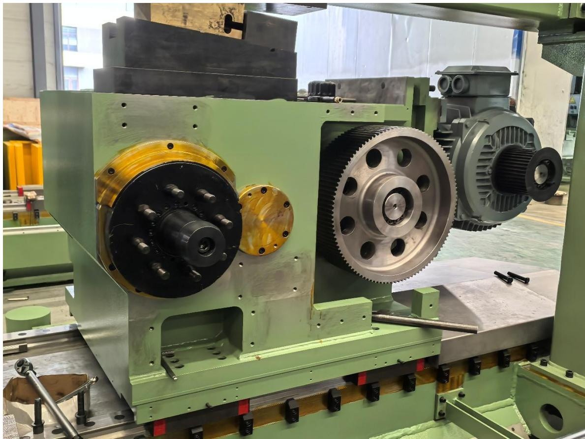
The Tooling box is a critical transmission component of the circular cold saw, engineered for high precision, durability, and stability. It is constructed from **Q345-B structural steel** through a **welded assembly**, followed by **stress-relief aging treatment** to eliminate internal stresses and ensure long-term structural integrity.
