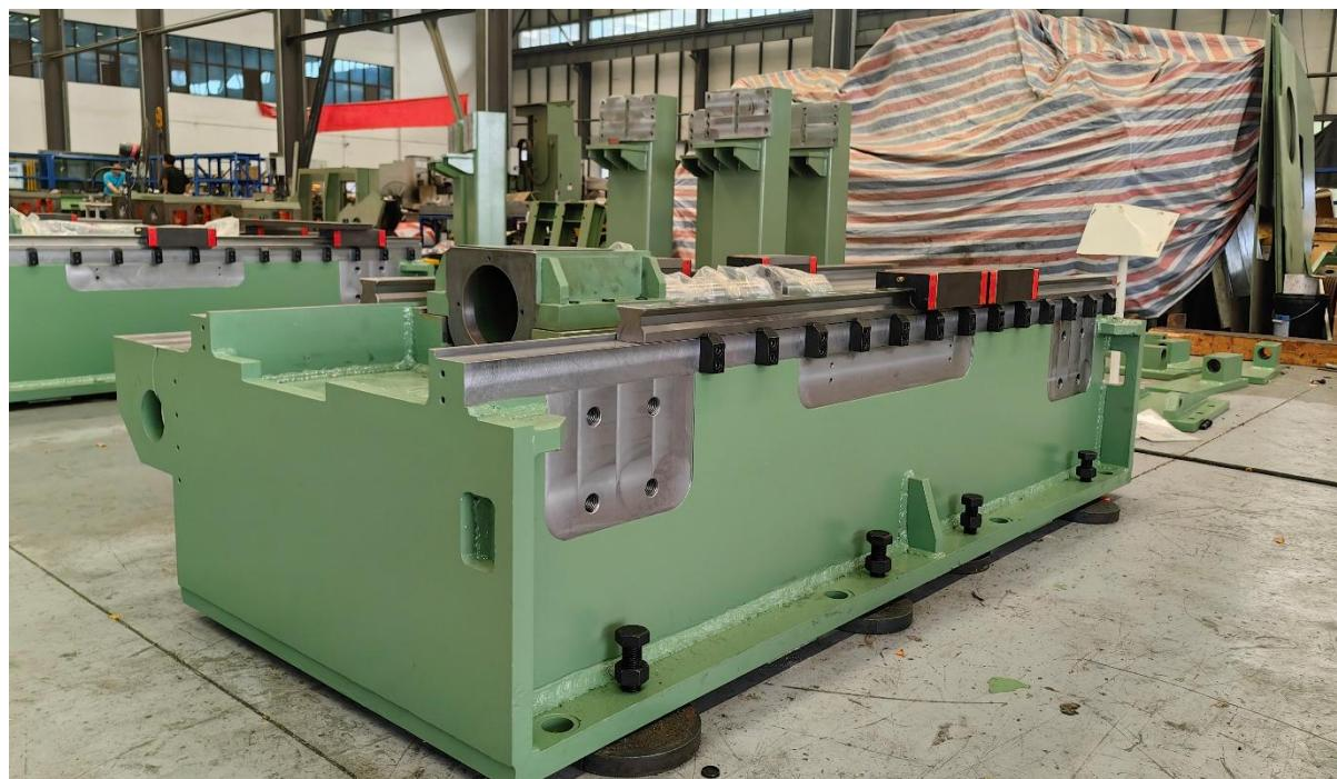
The machine bed, serving as the fundamental load-bearing structure, is fabricated from thick welded
