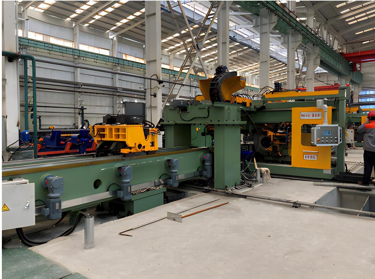
This high-performance **circular cold saw** is designed for precise and efficient cutting of metal billet and round bar Materials. Featuring a **horizontal cutting mechanism** and **carbide-tipped saw blades**, it delivers fast, accurate cuts suitable for a wide range of industrial applications.
