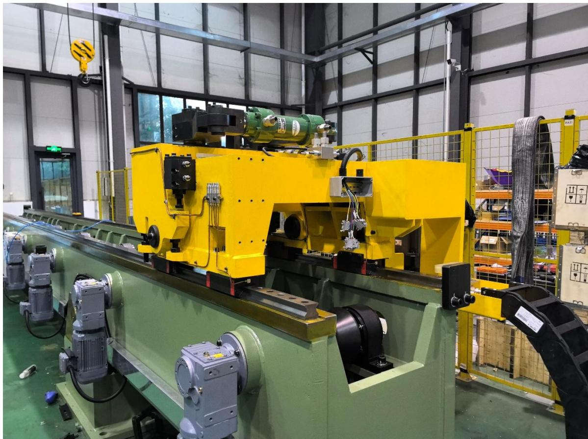
The feeding trolley is mounted on a vertically adjustable base and driven by a servo gear motor through a rack-and-pinion mechanism for precise linear movement along guide rails. Equipped with a hydraulic clamping arm to secure the billet, the lifting function of the base effectively prevents interference between the billet and the fixture during feeding, ensuring safe and stable operation.
