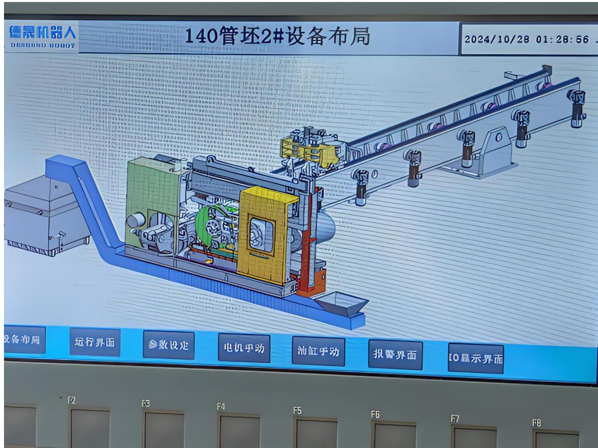
The HMI is developed using WinCC software, offering a visually appealing and intuitive interface that clearly displays the operational status of the equipment.
