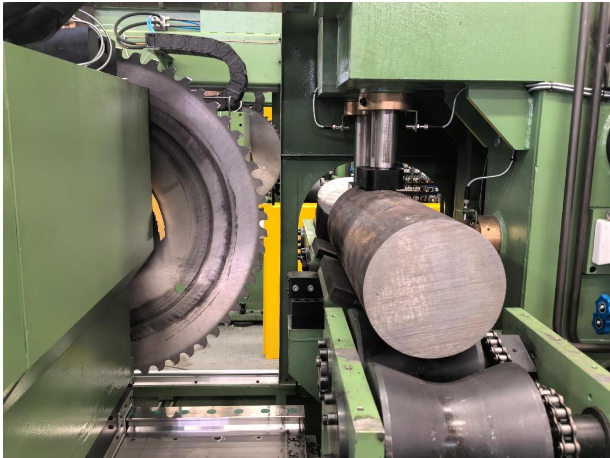
Each side of the saw blade is equipped with a hydraulic clamping unit, consisting of a horizontal clamp, a vertical clamp, and a clamping base.
